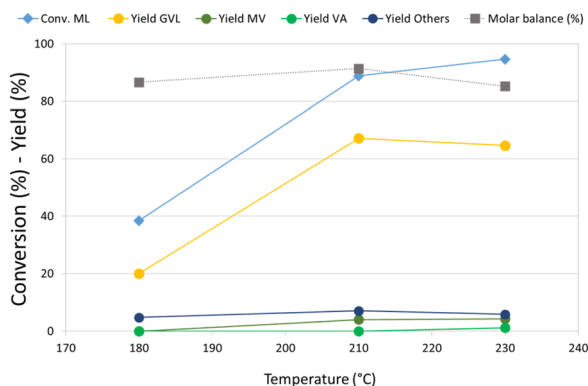
Fig. 1 Effect of temperature on ML hydrogenation over Re–O/HZSM-5. Reaction conditions: solvent free (ML neat), T = \text{variable} , P_{\text{H}_2} = 40 bar, t = 4 h, catalyst loading = 5 wt% [ m_{\text{cat}}/m_{\text{ML}} ]. Others = 2-MTHF, 4-HPA/E and unidentified products.
