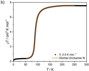
Fig. 4  $\chi T(T)$  dependence recorded for  ${f 1\cdot 4H_2O}$  at  $\mu_0 H_{\rm dc}=0.1\,{
