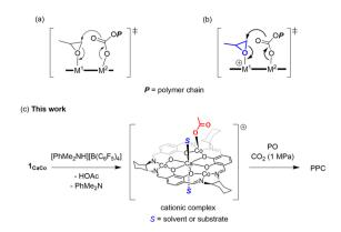
Scheme 1 Key transition state structures of (a) neutral multinuclear catalysts, (b) cationic multinuclear catalysts. (c) This work: alternating copolymerization of PO and  $\mathrm{CO}_2$  by cationic multinuclear species in the presence of anilinium salt.
