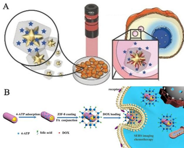
**Fig. 12** Schematic diagram of MOF-based SERS sensing platforms employed in bioimaging. (A) Schematic diagram of intracellular SERS imaging of Au nanostar@ZIF-8.<sup>107</sup> Reproduced with permission from John Wiley and Sons, copyright 2019. (B) Schematic diagram of the synthetic route and application instructions of Au@Ag nanorod@ZIF-8.<sup>108</sup> Reproduced with permission from Elsevier, copyright 2019.
