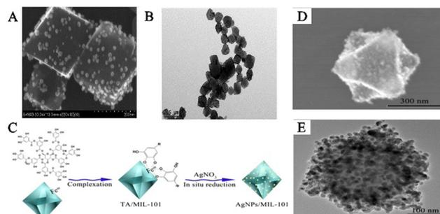
Fig. 6 The satellite PNPs/MOFs composites were synthesized. (A) SEM images of AgNPs/MIL-101(Cr). (B) TEM images of AgNPs/MIL-101(Cr).<sup>59</sup> Reproduced with permission from American Chemical Society, copyright 2015. (C) Schematic illustration of the preparation of AgNPs/MIL-101(Fe). (D) SEM images of AgNPs/MIL-101. (E) TEM image of AgNPs/MIL-101.<sup>60</sup> Reproduced with permission from the Royal Society of Chemistry, copyright 2016.
