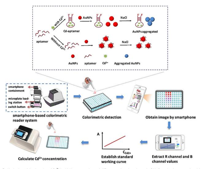
Fig. 5 Mechanism of the detection of Cd<sup>2+</sup> in drinking water using an AuNP-aptamer based sensing probe [this figure has been reproduced from ref. 56 with permission from Elsevier Sciences, copyright 2020].
