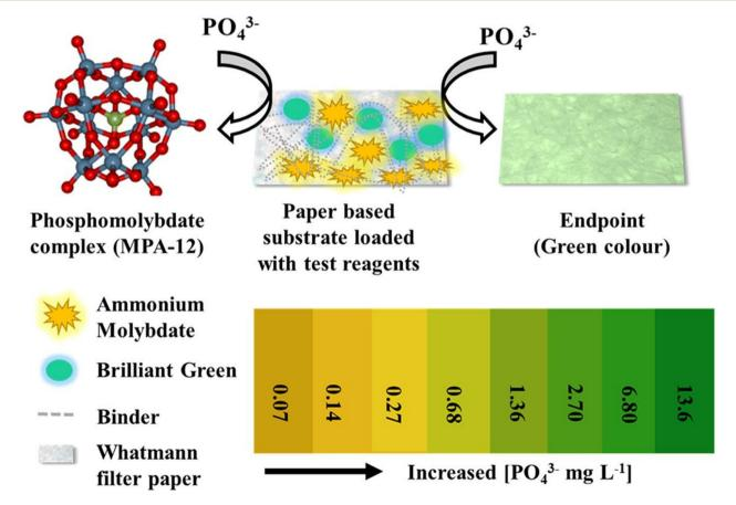
Fig. 10 A paper-based colorimetric sensor formulated with ammonium molybdate and BG for the detection of phosphate ion in drinking water [this figure has been reproduced from ref. 87 with permission from Elsevier Sciences, copyright 2021].
