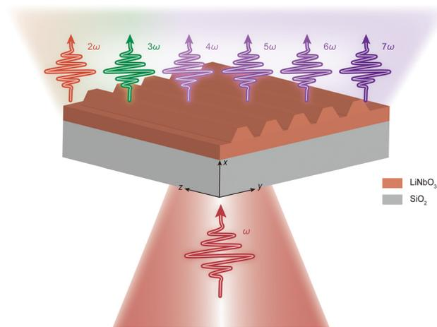
**Fig. 1** Schematic of HHG from a LiNbO<sub>3</sub> metasurface supporting guided-mode resonance. When the TE-polarized pump laser is normally incident from the substrate side, the nonlinear harmonic signals from the 2<sup>nd</sup> to 7<sup>th</sup> order are emitted in the transmission direction. The metasurface is composed of a LiNbO<sub>3</sub> grating whose optical axis is along the z-direction situated on a SiO<sub>2</sub>/quartz substrate.
