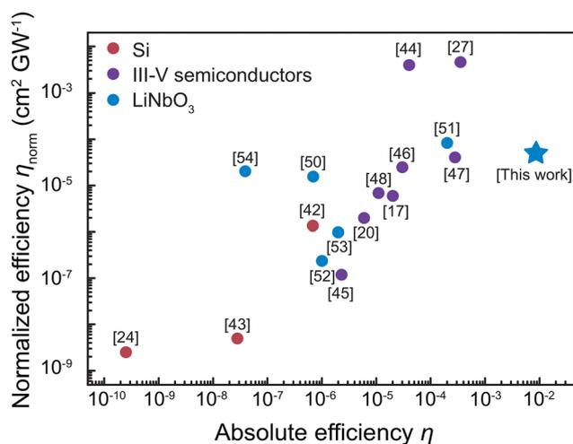
**Fig. 4** Comparison of SHG efficiency in Si, III–V semiconductors, and LiNbO<sub>3</sub> metasurfaces.
