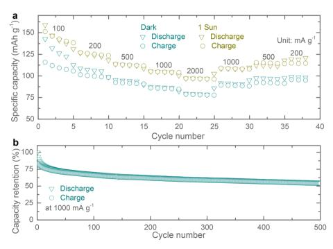
Fig. 5 (a) Rate specific capacity tests in the dark and 1 sun illuminated conditions. (b) Long term cycling stability test at 1000 mA  $g^{-1}$  in dark condition, showing specific capacity retentions of ~67% and ~55% after 100 and 500 cycles.
