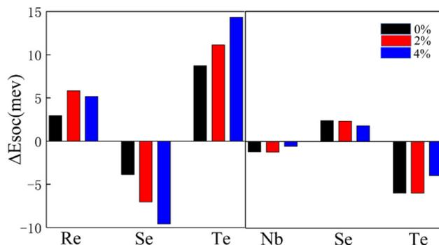
**Fig. 5** Atom-resolved localization of the SOC energy difference  $\Delta E_{\text{SOC}}$  in Janus ML-XSeTe. Black, red, and blue bars represent  $\Delta E_{\text{SOC}}$  of ML-XSeTe under 0%, 2%, and 4% tensile strain, respectively.
