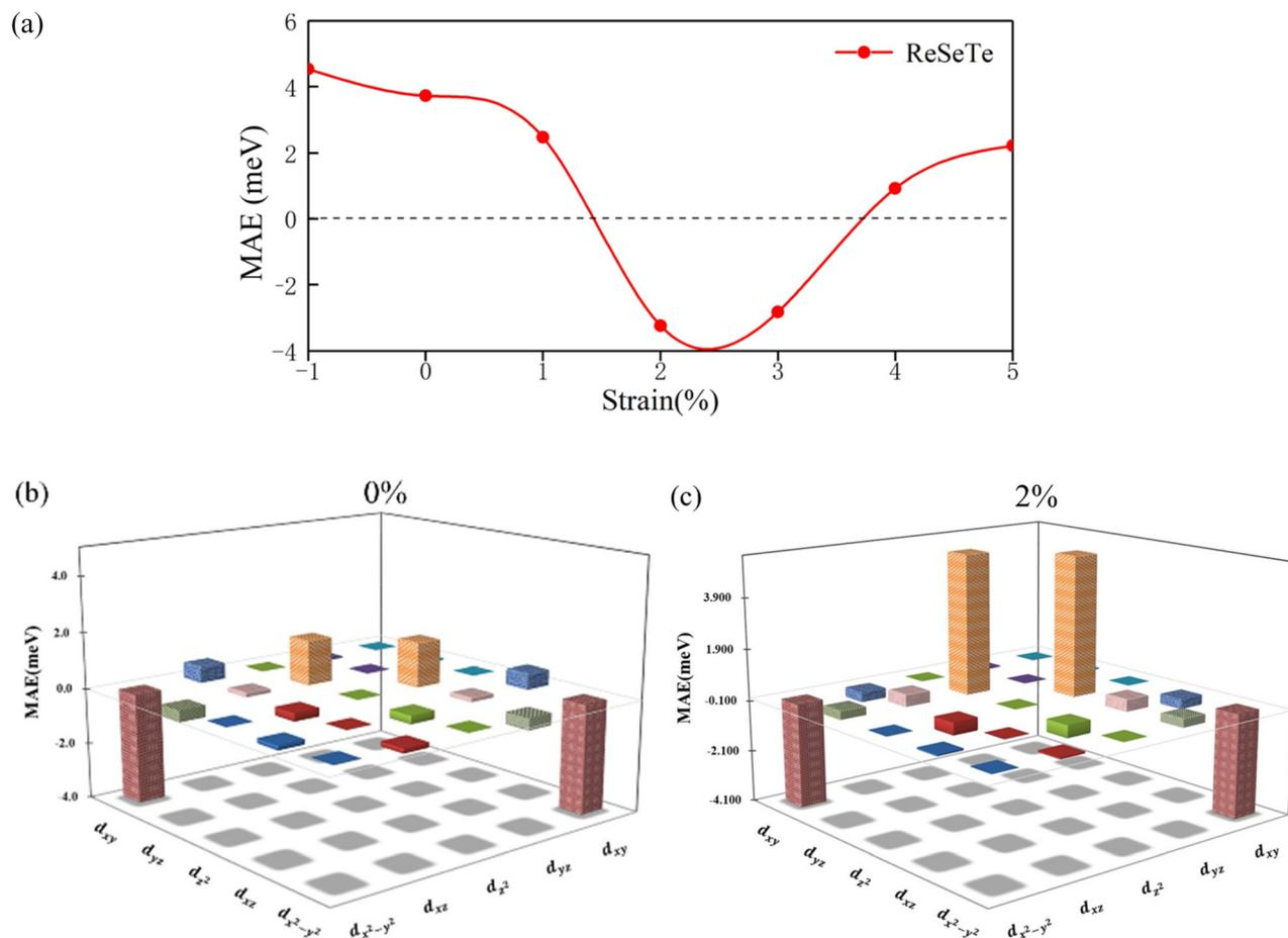
**Fig. 4** (a) Single-ion anisotropy  $K$  as a function of strain in Janus ML–ReSeTe. (b) and (c) MAE contributions from 5p orbital hybridization of Re in Janus ML–ReSeTe under 0 and 2% tensile strain, respectively.
