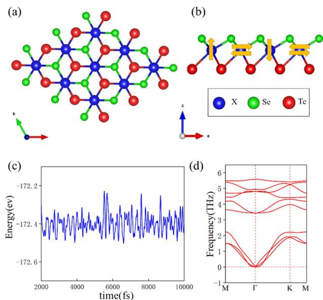
**Fig. 1** The top (a) and side (b) views of the crystal structure and the phonon spectra for ML-XSeTe ( $X = \text{Nb, Re}$ ). The yellow vectors in (b) indicate the two spin configurations with opposite chirality used to extract the IP DMI parameters. (c) The molecular dynamics simulation of ML-ReSeTe. (d) Phonon spectrum of ML-ReSeTe.
