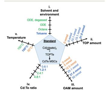
Fig. 1 Diagram showing different reaction conditions explored in this work. Standard conditions are highlighted in bold. The conditions that produce MSCs, a mixture of MSCs and QDs, and no MSCs are labeled in blue, green, and orange, respectively.
