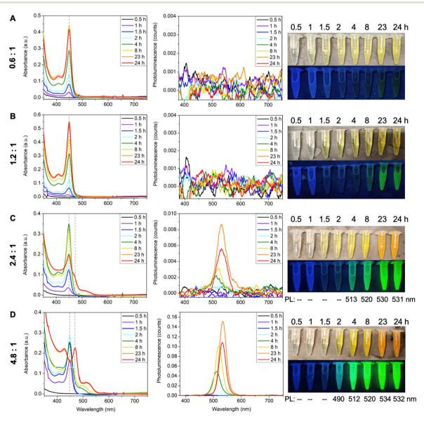
Fig. 4 Effect of Cd: Te ratio on CdTe MSC formation. The amount of TOPTe is set to 1 mmol, while the Cd(oleate)<sub>2</sub> is varied from (A) 0.6 mmol, (B) 1.2 mmol, (C) 2.4 mmol, and (D) 4.8 mmol. The reactions are monitored by absorption, emission, and photos of aliquots under ambient light and UV light.
