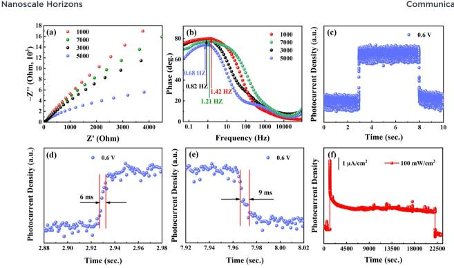
Fig. 6 (a) EIS spectra, (b) Bode plots of NbSe<sub>2</sub>/Nb<sub>2</sub>O<sub>5</sub> photoelectrodes covered with different sizes of nanosheets, (c) response time including (d) rise time  $(t_r)$  and (e) fall time  $(t_f)$ , and (f) long-term stability measurement.
