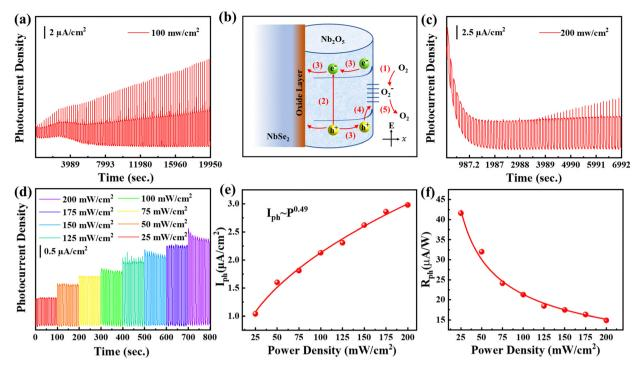
Fig. 7 (a) Long cycling stability measurement in a low oxygen environment, (b) OSPC mechanism, (c) long cycling stability measurement in enough oxygen environment, (d) light intensity-dependent photocurrent density, and (e)  $I_{ph}$  and (f)  $R_{ph}$  values extracted from (d).
