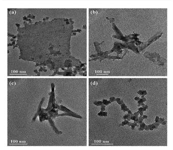
Fig. 2 TEM images of NbSe<sub>2</sub> nanosheets under the centrifugation speed of (a) 1000 rpm, (b) 3000 rpm, (c) 5000 rpm, and (d) 7000 rpm.
