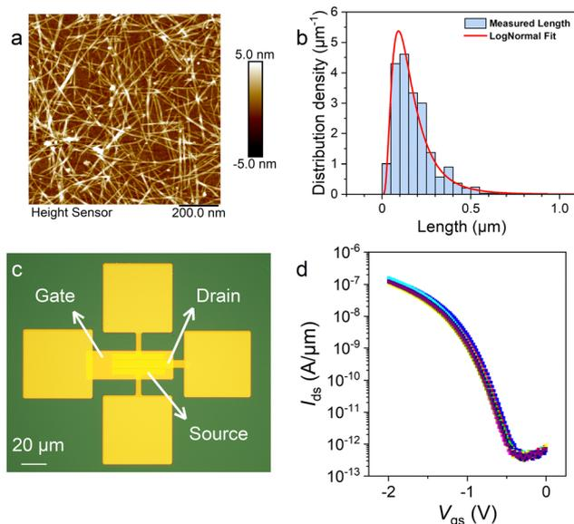
**Fig. 5** Characterizations of the FETs fabricated by SWCNTs synthesized from coal. (a) AFM image of the SWCNT membrane on the Si substrate, size: 1  $\mu\text{m}$ . (b) Length distribution of the SWCNTs sorted by PCz. (c) Optical photograph of the FET, objective: 50 $\times$ . (d) Transfer characteristic curves of 10 FETs fabricated by the semiconducting SWCNTs sorted by PCz.
