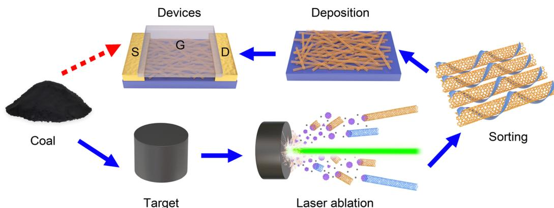
**Fig. 6** Scheme of the strategy of transforming natural coal into electronic devices.
