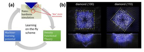
Fig. 1 Learning on-the-fly on atomic environments for the simulation of nanoindentation of covalent bulk materials (reprinted from ref. 46, copyright 2022, American Chemical Society).
