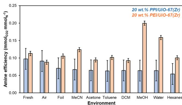
Fig. 4 Amine efficiencies ( $\text{mmol}_{\text{CO}_2} \text{ mmol}_{\text{N}}^{-1}$ ) determined from 1 h  $\text{CO}_2$  uptakes at 308 K from simulated flue gas for 20 wt% PPI/UiO-67(Zr) (blue) and 20 wt% PEI/UiO-67(Zr) (orange) after 7 days of exposure to each solvent environment. Amine contents are based on molecular weights of  $400 \text{ g mol}^{-1}$  for PPI (77% primary and secondary amines) and  $800 \text{ g mol}^{-1}$  for PEI (77% primary and secondary amines).<sup>36,37</sup>
