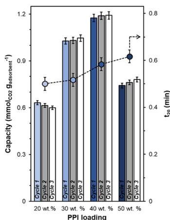
Fig. 2 Mass-normalized  $\text{CO}_2$  capacities for varying weight percentages (20–50) of PPI supported on UiO-67(Zr) for three 1 h uptake cycles at 308 K from simulated flue gas with 2 h regeneration steps at 383 K under 40  $\text{mL min}^{-1}$  Ar flow in between cycles.  $t_{20}$  (circles) are times to reach 20% of equilibrium  $\text{CO}_2$  uptakes.
