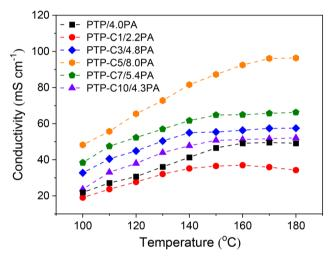
Fig. 4 Proton conductivities of the PTP and PTP-Cx membranes doped in 85 wt% PA solution at 60 °C.
