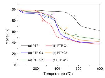
Fig. 3 TGA curves of (a) PTP and (b-f) PTP-Cx membranes in a N<sub>2</sub> atmosphere at a heating rate of 10 °C min<sup>-1</sup>.
