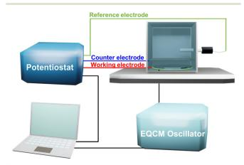
Fig. 2 Scheme of EQCM system.
