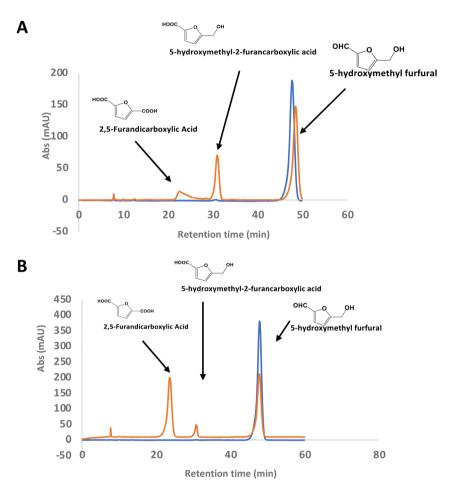
Fig. 4 Conversion of HMF to FDCA by *R. jostii* RHA1 glycolate oxidase. (A) Small scale (1 ml) conversion of 2 mM HMF by 90 μg Rj GlOx; (B) large scale (100 ml) conversion of 200 mg (16 mM) HMF by 9 mg Rj GlOx. Orange, reaction mixture containing enzyme; blue, control reaction lacking enzyme. All bioconversions incubated in 50 mM phosphate buffer pH 7.5 for 24 h at 30 °C.
