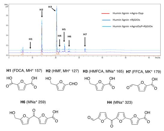
Fig. 8 Total ion chromatogram of products from bioconversion of Avantium humins by AgroDyP and RjGlOx. Structures for H1-H3 and H7 confirmed by co-elution with authentic standards, structures for H4 and H6 based on predicted humin structure.<sup>30</sup>
