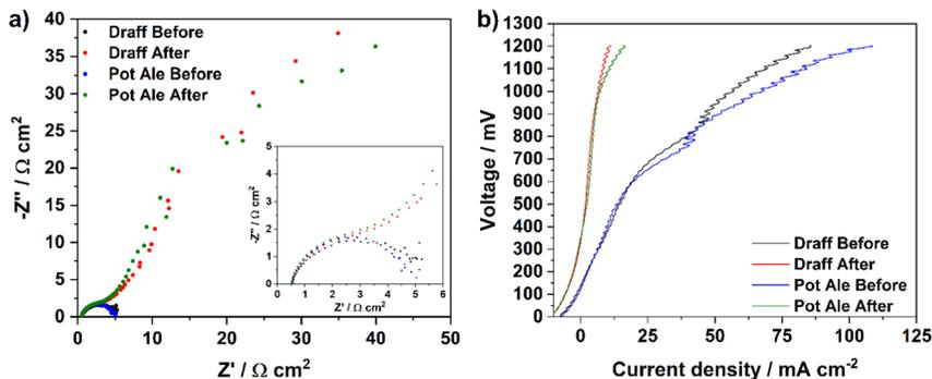
Fig. 12 Complex-plane EIS for PEMEC2 operating with digested draff (D4)–PMA and pot ale (PA2)–PMA anolyte solutions, collected at 850 mV before and after chronoamperometry experiments, and (b)  $V-I$  curves for PEMEC2 operating with the same anolyte solutions, before and after chronoamperometry experiments at 80 °C using  $\text{H}_2\text{SO}_4$  as a catholyte.
