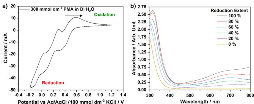
Fig. 5 (a) CV plot of a 300 mmol dm<sup>-3</sup> solution of H<sub>3</sub>[PMo<sub>12</sub>O<sub>40</sub>]·25.1H<sub>2</sub>O (in DI H<sub>2</sub>O), collected between -200 mV and 1200 mV *vs.* a Ag/AgCl reference electrode and (b) UV-visible spectra of PMA solution reduced by 0, 20, 40, 60, 80 and 100%, with respect to the first two-electron process, through chronoamperometric experiments.
