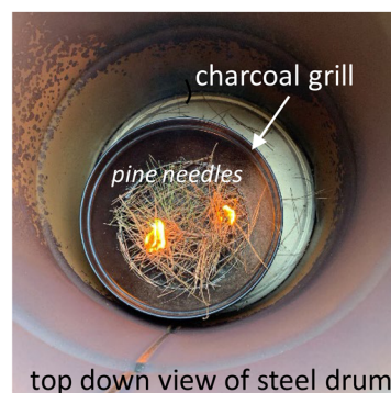
Fig. 1 (A) Sampling and wildfire locations, and the smoke plumes and wildfire hotspots from the Silverado Fire (on October 26, 2020) as viewed by the Moderate Resolution Imaging Spectroradiometer (MODIS). Laboratory combustion experiments with (B) pyrolysis and (C) flaming combustion of pine needles.
