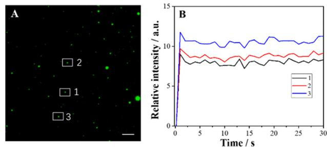
Fig. 4 (A) ECL image of  $\text{Co}_3\text{O}_4$  at ITO slides; (B) the fluctuation of ECL intensity at three particles labeled as 1, 2 and 3 in (A). The exposure time was 500 ms; the applied potential was 1 V. Scale bar: 5  $\mu\text{m}$ .
