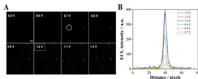
**Fig. 2** (A) ECL image of  $\text{Co}_3\text{O}_4$  at the ITO slides with different applied potentials; the exposure time was 1 s. (B) The luminescence intensity across the particle circle in image A. Scale bar: 5  $\mu\text{m}$ .
