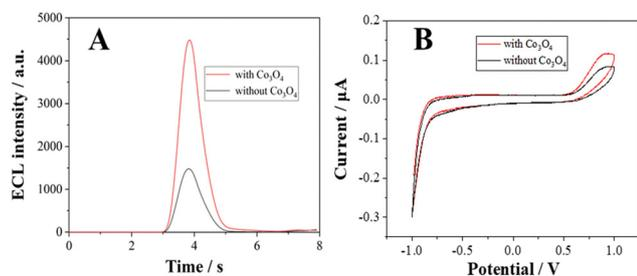
**Fig. 1** (A) ECL profiles and (B) CV curves of the L012- $\text{H}_2\text{O}_2$  system at the ITO surface with and without  $\text{Co}_3\text{O}_4$ . Working solution: 10 mM PBS containing 200  $\mu\text{M}$  L012. Scan range:  $-1.0$  to  $1.0$  V, scan rate:  $0.1$  V  $\text{s}^{-1}$ , PMT voltage: 600 V.
