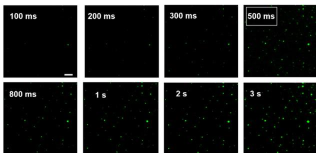
Fig. 3 ECL image of  $\text{Co}_3\text{O}_4$  at ITO slides with different exposure times; the applied potential was 1 V. Scale bar: 5  $\mu\text{m}$ .
