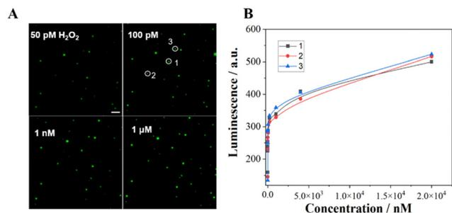
Fig. 5 (A) ECL image of  $\text{Co}_3\text{O}_4$  at ITO slides with different concentrations of  $\text{H}_2\text{O}_2$ ; the exposure time was 500 ms, and the applied potential was 1 V. (B) Correlation between the luminescence of three particles and the concentration of  $\text{H}_2\text{O}_2$ . Scale bar: 5  $\mu\text{m}$ .
