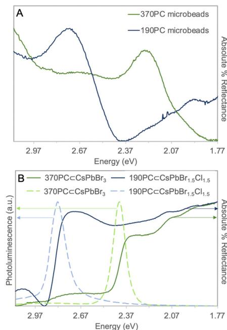
**Fig. 1** (A) Absolute % reflectance of 370PC and 190PC microbeads and (B) normalized optical data for 370PC $\subset$ CsPbBr<sub>3</sub> and 190PC $\subset$ CsPbBr<sub>1.5</sub>Cl<sub>1.5</sub> hybrids ( $\lambda_{ex}$  = 365 nm).
