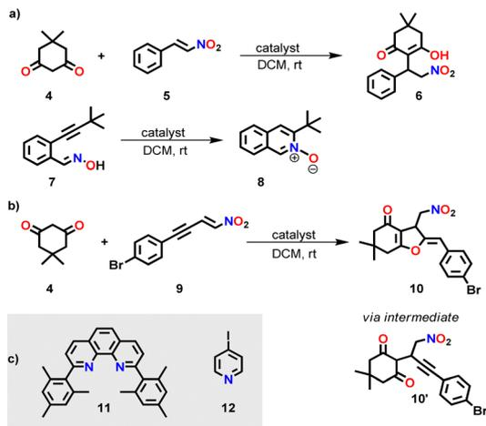
**Scheme 2** (a) Parallel one-pot base-catalyzed Michael addition and silver(i)-catalyzed cyclization. For catalyst(s), see Tables 1 and 2. (b) Sequential Michael addition/hydroalkoxylation reaction (for mechanism, see ESI,† Scheme S4).<sup>17</sup> (c) Further ligands used in this study.
