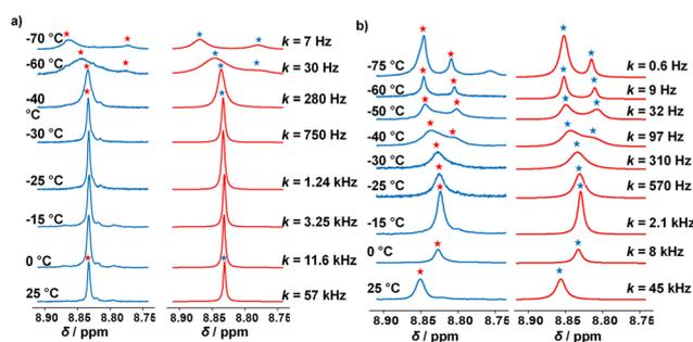
Fig. 3 Experimental (left) and simulated (right) partial VT  $^1\text{H}$  NMR spectra ( $\text{CD}_2\text{Cl}_2$ , 600 MHz) of (a)  $[\text{Ag}_3(\mathbf{1})(\mathbf{2})]^{3+}$  and (b) of  $[\text{Ag}_3(\mathbf{1})(\mathbf{2})(\mathbf{3})]^{3+}$ .
