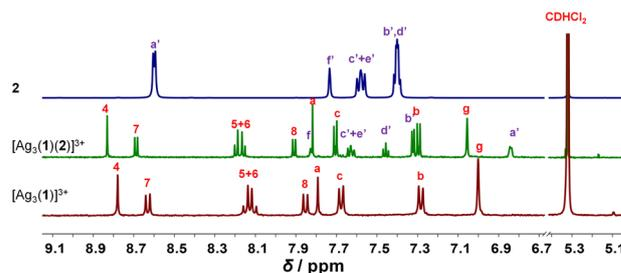
**Fig. 1** Partial <sup>1</sup>H NMR (600 MHz, CD<sub>2</sub>Cl<sub>2</sub>, 298 K) of silver(i)-loaded deck [Ag<sub>3</sub>(**1**)(**2**)<sub>3</sub>]<sup>3+</sup>, slider-on-deck [Ag<sub>3</sub>(**1**)(**2**)<sub>3</sub>]<sup>3+</sup> and biped **2**.
