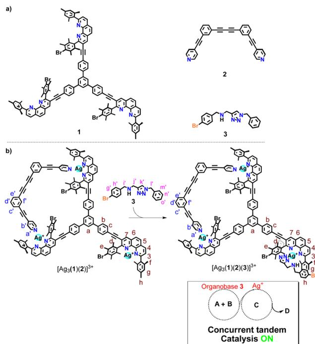
**Scheme 1** (a) Chemical structure of ligands **1–3**. (b) Transformation of the three- into the four-component dual-catalyst machinery. Both organobase **3** and the silver(I) centers are liberated due to the sliding motion in  $[Ag_3(1)(2)(3)]^{3+}$ , which enables concurrent tandem catalysis. A & B represent the substrates, C denotes the intermediate product and D the final product of the concurrent tandem reaction.
