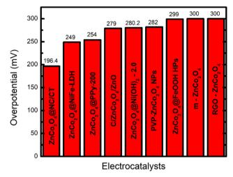
Fig. 23 The top 9 electrocatalysts based on ZnCo<sub>2</sub>O<sub>4</sub> for the OER that presented an overpotential  $\leq$ 300 mV ( $\eta_{10} \leq$  300 mV).
