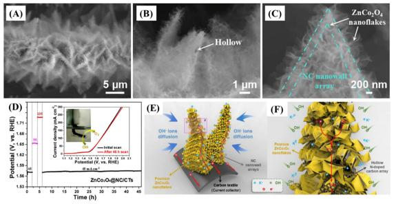
Fig. 22 (A-C) SEM images of  $ZnCo_2O_4@NC/CT$ . (D) Stability measurements of  $ZnCo_2O_4@NC/CT$  at different current densities and (E and F) schematic illustration of the ZnCo<sub>2</sub>O<sub>4</sub>@NC/CT electrode. Reproduced with permission.<sup>138</sup> Copyright © 2019 Published by Elsevier B.V.
