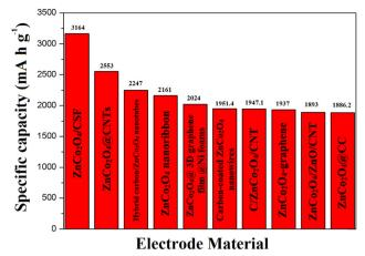
Fig. 17 The ZnCo<sub>2</sub>O<sub>4</sub> electrode materials with the top 10 highest first specific capacity in LIBs
