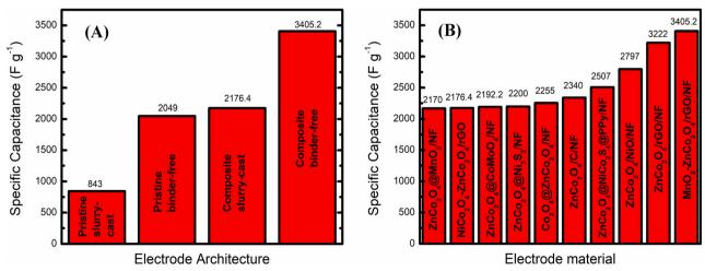
Fig. 13 (A) Best specific capacitance for each ZnCo<sub>2</sub>O<sub>4</sub>-based electrode type: pristine slurry-cast; pristine binder-free; composite slurry-cast and composite binder-free (ref. 11, 26, 58 and 62, respectively). (B) Top 10 specific capacitances delivered by ZnCo<sub>2</sub>O<sub>4</sub>-based electrodes (ref. 62, 43, 38, 90, 84, 67, 75, 79, 58 and 89, respectively)
