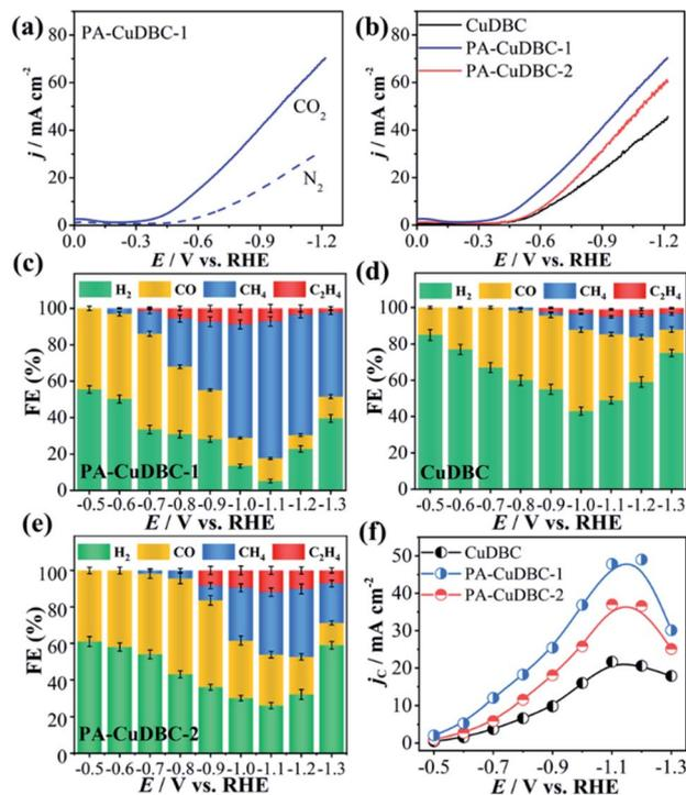
Fig. 3 (a) LSVs of PA-CuDBC-1 in  $N_2$  or  $CO_2$ -saturated 0.5 M  $KHCO_3$  electrolyte; (b) LSVs of the three samples in  $CO_2$ -saturated 0.5 M  $KHCO_3$  electrolyte; product distribution and Faraday efficiencies with error bars of (c) PA-CuDBC-1, (d) CuDBC and (e) PA-CuDBC-2, and error bars correspond to the standard deviation of three independent measurements; (f) partial current densities of carbon-containing products.
