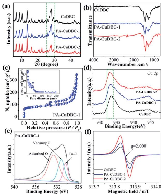
Fig. 2 (a) XRD patterns and (b) FT-IR spectra of the three samples; (c)  $N_2$  sorption isotherms of PA-CuDBC-1, inset shows the pore size distribution; (d) Cu 2p XPS spectra of the three samples; (e) O 1s XPS spectra of PA-CuDBC-1; (f) EPR profiles of the three samples.
