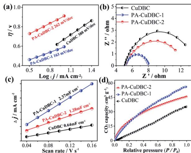
Fig. 4 (a) Tafel plots, (b) EIS and (c) ECSA of the three samples; (d) CO<sub>2</sub> adsorption capacity of the three samples.
