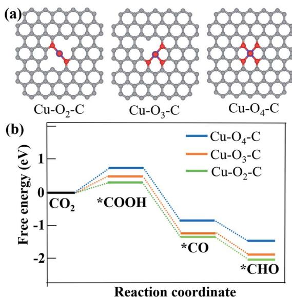
Fig. 5 (a) Optimized structures of  $Cu-O_2-C$ ,  $Cu-O_3-C$  and  $Cu-O_4-C$  moieties; (b) free energy diagram of  $CO_2$  to  $*COOH$ ,  $*CO$  and  $*CHO$  intermediates on  $Cu-O_2-C$ ,  $Cu-O_3-C$  and  $Cu-O_4-C$  structures.
