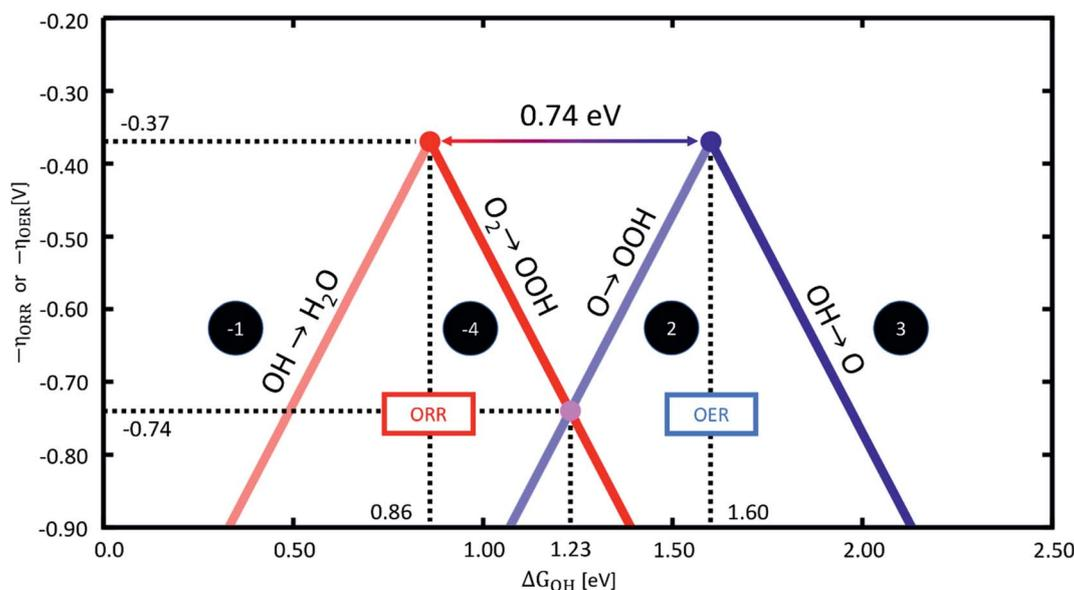
Fig. 1 Sabatier-type activity plots based on scaling relations for the OER (right) and ORR (left) as a function of  $\Delta G_{\text{OH}}$ . They are based on an energetic separation between \*OOH and \*OH of 3.20 eV, see Sections S1 and S2 in the ESI.† The most representative potential-limiting steps are noted in each case and have been determined statistically<sup>13,18</sup> from eqn (1)–(4) for the OER and the reverse equations for the ORR.
