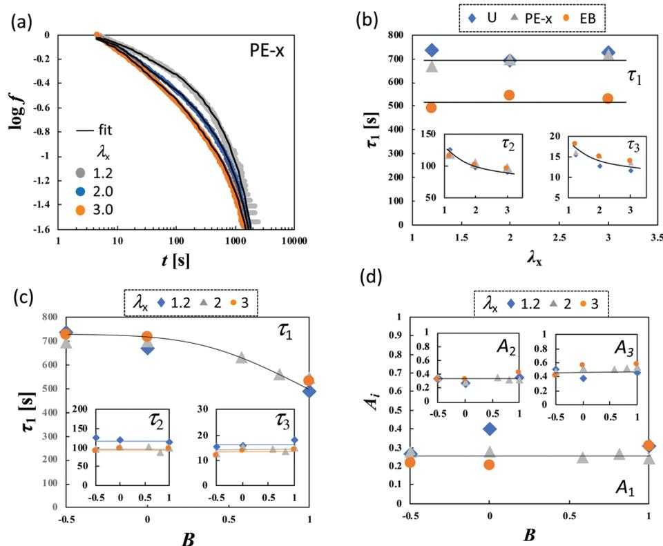
Fig. 6 (a)  $\log f - \log t$  curves for planar extension in  $x$ -direction with various values of  $\lambda_x$  for HGG63-0. The black solid lines represent the fitted curves of eqn (2). (b) Dependence of  $\tau_i$  ( $i = 1, 2$ , and  $3$ ) on  $\lambda_x$  in various types of stretching, (c) Dependence of  $\tau_i$  ( $i = 1, 2$ , and  $3$ ), and (d)  $A_i$  ( $i = 1, 2$ , and  $3$ ) on the anisotropy of the imposed strain field ( $B$ ) for various values of  $\lambda_x$  for HGG63-0.
