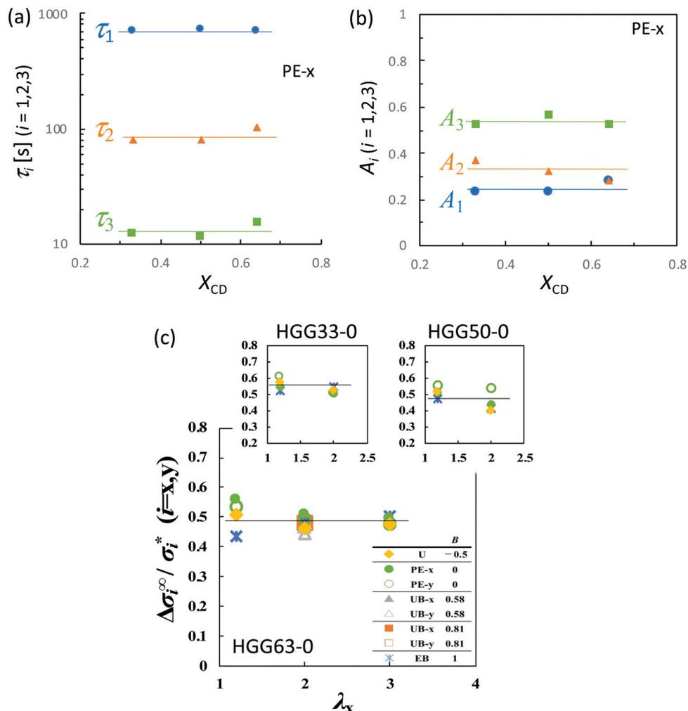
Fig. 7 (a) Relaxation times,  $\tau_i$  ( $i = 1, 2$ , and  $3$ ) and (b) relaxation strengths,  $A_i$  ( $i = 1, 2$ , and  $3$ ) as a function of  $X_{CD}$  for  $\sigma_x$  in planar extension. (c) Total stress relaxation ( $\Delta\sigma_i^\infty$ ) in several types of stretching as a function of  $\lambda_x$  for the HG gels with various values of  $X_{CD}$ .  $\Delta\sigma_i^\infty$  is reduced by the initial stress ( $\sigma^*$ ) in each deformation.
