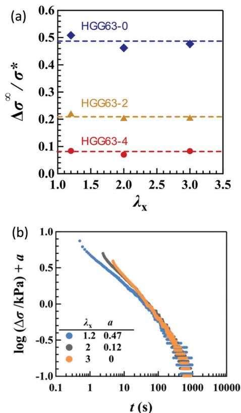
Fig. 8 (a) Total stress relaxation ( $\Delta\sigma^\infty$ ) in uniaxial stretching as a function of  $\lambda_x$  for the HG gels with  $X_{CD} = 0.63$  and various concentrations of covalent cross-links. (b) Failure of the superposition of  $\log \Delta\sigma - \log t$  curves for uniaxial stretching with various values of  $\lambda_x$  by vertical shift with a factor of  $a$  for HGG63-2.
