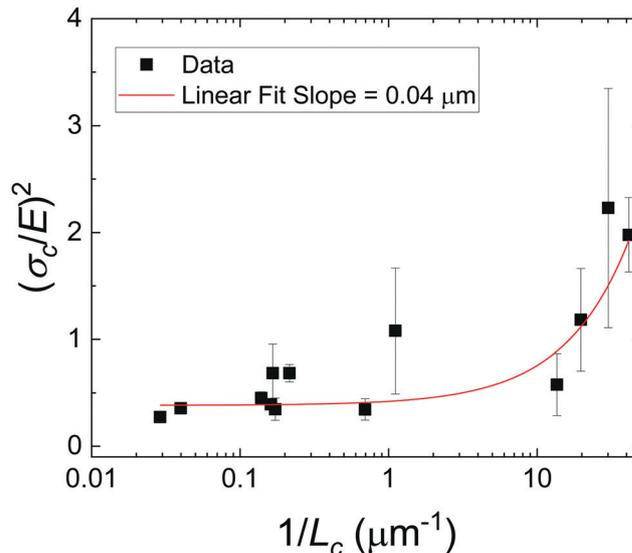
Fig. 5 Plot showing  $(\sigma_c/E)^2$  against  $1/L_c$  for the composite hydrogels used in this study. Note that the x-axis is plotted on log scale. The slope on this plot,  $0.04 \mu\text{m}$ , is well below the elastofracture length of these materials and no significant transition is observed. This likely indicates that the assumption that  $a = L_c$  in the absence of a macroscopic notch is incorrect.
