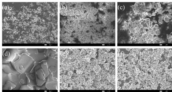
Fig. 4 Representative SEM images: Poly(VBS-DVB) was formed by different initiator dosage ((a) 1 wt%, (b) 3 wt%, (c) 10 wt%); (d) VBS; (e) Poly(VBS-DVB)HSO<sub>4</sub> (3 wt% initiator dosage); (f) recovered Poly(VBS-DVB)HSO<sub>4</sub> (3 wt% initiator dosage).
