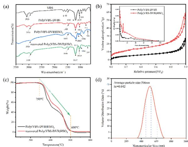
Fig. 2 (a) FT-IR spectra of VBS, Poly(VBS-DVB), Poly(VBS-DVB)HSO<sub>4</sub> and recovered Poly(VBS-DVB)HSO<sub>4</sub>; (b) N<sub>2</sub> adsorption–desorption isotherms and pore size distribution curves of Poly(VBS-DVB) and Poly(VBS-DVB)HSO<sub>4</sub>; (c) TG curves of Poly(VBS-DVB)HSO<sub>4</sub> and recovered Poly(VBS-DVB)HSO<sub>4</sub>; (d) nanoparticle size distribution diagram of 506 nm.
