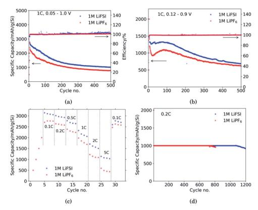
Fig. 1 Galvanostatic cycling tests comparing half cells with 60 wt% Si electrodes cycled in 1 M LiFSI (blue) or 1 M LiFF<sub>6</sub> (red). (a) Galvanostatic cycling in voltage range 0.05-1.0 V, (b) galvanostatic cycling in voltage range 0.12-0.9 V, (c) rate capability in voltage range 0.05-1.0 V, (d) galvanostatic cycling at 0.2C with lithiation of silicon limited to  $1000 \text{ mA h g}^{-1}$  and delithiation to 1.0 V.
