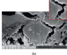
Fig. 2 Comparison of cross sections in Si electrodes after 10 cycles in (a) 1 M LiFSI and (b) 1 M LiPF<sub>6</sub>. A layer of carbon has been coated on the electrode surface to protect the electrode structure beneath from the ion beam during sputtering.
