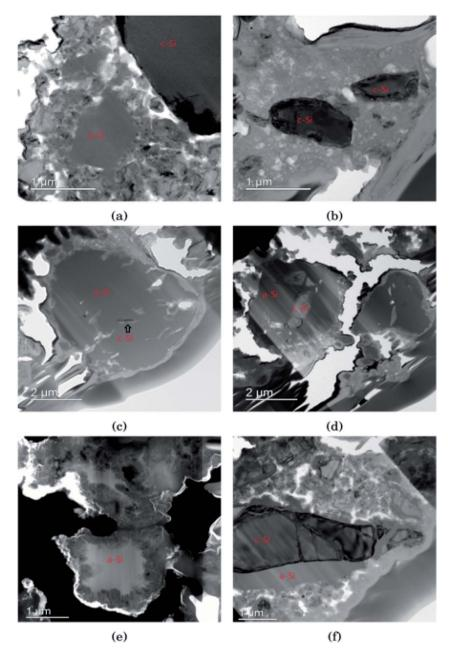
Fig. 3 Bright field TEM images after the first cycle in (a) LiFSI and (b) LiPF<sub>6</sub> (c) after 10 cycles in LiFSI and (d) LiPF<sub>6</sub> (e) high angle annular dark field scanning transmission electron microscopy image of LiFSI after 50 cycles and (f) bright field TEM image of LiPF<sub>6</sub> after 50 cycles.
