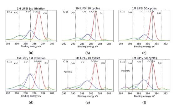
Fig. 7 C 1s spectra for Si electrodes cycled to 1st lithiation, cycle 10 and cycle 50 in LiFSI (a-c) respectively, and in LiPF<sub>6</sub> (d-f) respectively.
