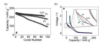
Fig. 7 (a) Capacity retention and (b) initial charge/discharge of hard-carbon electrodes cycled in 1 mol dm $^{-3}$  NaPF $_6$  PC-based electrolyte containing 0, 0.5, 1, and 2 vol% of FEC concentration.  $^{23}$  Copyright 2016, John Wiley & Sons, Inc.
