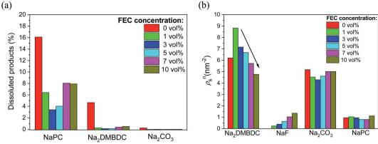
Fig. 8 FEC concentration dependence (a) on the numbers of dissoluted SEI products, and (b) on the surface number densities  $(\rho_s^n)$  of the SEI film products.
