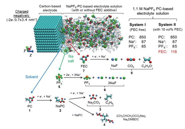
Fig. 1 Model simulation system and reaction schemes in the PC-based electrolyte. (cyan: C, red: O, white: H, orange: P, green: F, blue: Na<sup>+</sup>).
