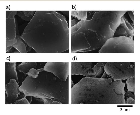
Fig. 4 SEM images for hard-carbon electrodes; (a) pristine, and (b-d) after the first reduction-oxidation cycle test in PC-based electrolyte solutions (b) without and (c and d) with (c) 2 vol% and (d) 10 vol% FEC at a rate of 25 mA  $g^{-1}$  in the coin-type Na cells.<sup>70</sup> Copyright 2014, Elsevier B. V.
