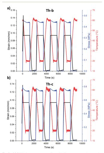
Fig. 2 (a) DMA shape memory cycling of bulk-cast rectangular samples made with Th-b resin. Over four cycles, 97% shape recovery is visible in the first cycle, and 100% shape recovery for remaining cycles. (b) DMA shape memory cycling of bulk-cast rectangular samples made with Th-c resin. Similarly, Th-c samples show 97% shape recovery in the first cycle, and 100% shape recovery for the three remaining cycles. Stress (blue), strain (black) and temperature (red, secondary axis) are displayed in
