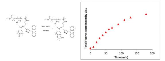
Fig. 1 Evolution of total fluorescence over time when a polymer decorated with an anthracene chromophore and nitroxide moiety is heated at 100 °C in a degassed solution of toluene containing 2.5 equivalents of AIBN. Figure reproduced with permission from ref. 37. Copyright, Royal Society of Chemistry, 2015.
