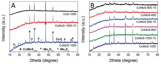
Fig. 2 XRD patterns of (A) CoS-1000, CoMoS-1000-10 and CoMoS-1000 and (B) samples derived from Mo-Z67-D at 600, 800, and 1000 °C at a heating ramp rate of 10 and 2 °C min<sup>-1</sup> respectively.
