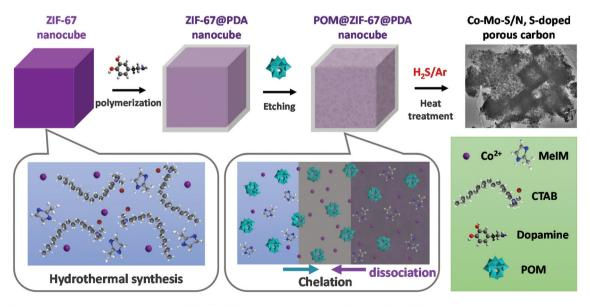
Scheme 1 Diagram of the synthesis of the POM@ZIF-67@PDA precursor and bimetallic Co-Mo-S/C composites.
