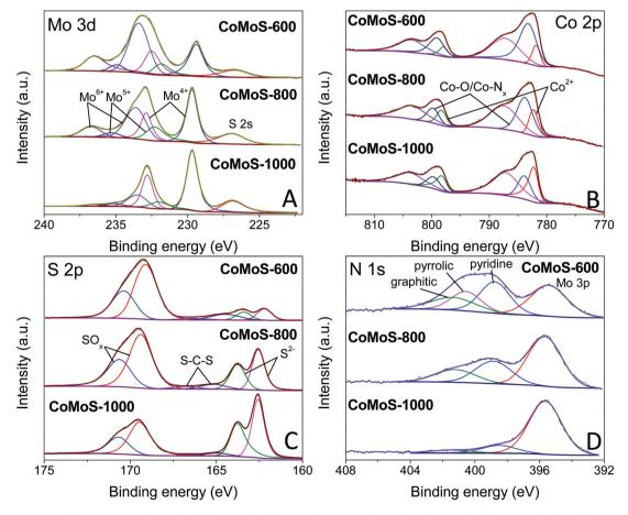
High-resolution XPS spectra of (A) Mo 3d, (B) Co 2p, (C) S 2p and (D) N 1s for CoMoS-600, CoMoS-800 and CoMoS-1000.
