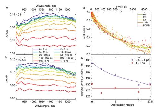
Fig. 3 Transient absorption spectra for neat AgBiS<sub>2</sub> films after (a) 0 h and (b) 27.5 h degradation following a 700 nm excitation. (c) Evolution in time of the normalised TA PIA signal for all films. (d) Centre of mass of PIA signal as a function of degradation time for early and late pump-probe time
