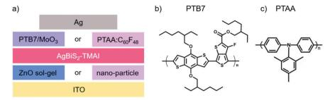
Fig. 1 Structure of devices and materials. (a) Architecture of the studied solar cells. The HTL consists either of PTB7/MoO<sub>3</sub> or PTAA: $C_{60}F_{48}$  and the molecular structure is shown in (b) and (c) for the polymers, respectively. The ETL was made from ZnO but either in a sol-gel thin film or as nanoparticles, resulting in overall four combinations which were examined.
