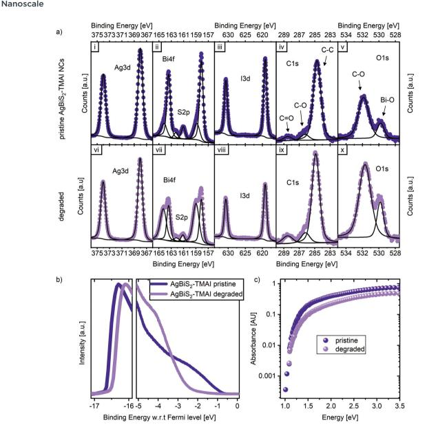
Fig. 5 The degradation of AgBiS<sub>2</sub>-TMAI NCs. (a) XPS data of a pristine film in the top row, bottom row presents the state after 24 h of dry air and sunlight exposure. The scale is arbitrary but the same for each orbital. (b) UPS data for a pristine and 17 h degraded AgBiS<sub>2</sub>-TMAI film on ITO. (c) PDS measurement of the absorption of a pristine and 24 h degraded film.
