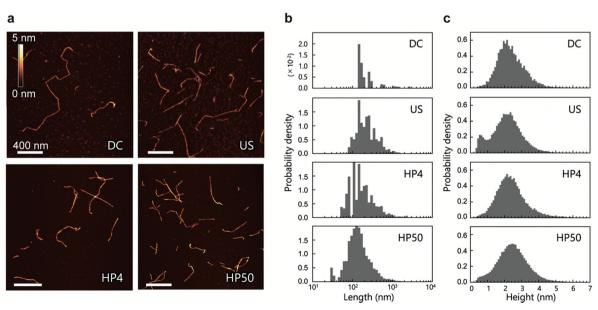
Fig. 1 Morphology of CNFs. (a) Typical AFM images of CNF samples: DC, US, HP4, and HP50. (b) Length distributions of CNFs. For overlapped and aggregated CNFs, total length was calculated as the length. (c) Height distributions obtained from all pixels along the centerlines of the CNFs.
