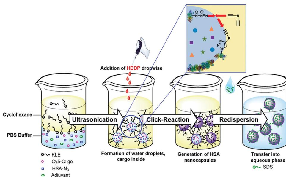
Fig. 1 Multicomponent encapsulation into protein nanocarriers through interfacial azide–alkyne crosslinking in inverse miniemulsion.
