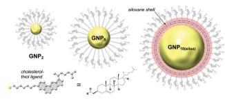
Fig. 2 Studies focusing on the effects of core diameter and presence (absence) of a chiral bias during GNP formation. GNP2 and GNP5 (the subscript number indicating the average core diameter) are capped with cholesterol-thiol ligands; GNP<sub>10(silox)</sub> is capped with a siloxane shell using 3-mercaptopropyltrimethoxysilane (MPS) that is further functionalized with cholesterol. Reproduced from and adapted with permission from ref. 19 - Copyright (2014), American Chemical Society.
