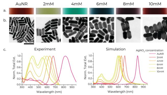
Fig. 1 Synthesis of Au/AgNRs with varying shell thickness. (a) Variation of colour of Au/AgNR suspensions grown with different concentrations of  $Ag^+$  ions. (b) Transmission electron micrographs of Au/AgNRs with Ag shells of different thicknesses. The concentration of  $Ag^+$  in the growth solution is shown at the top. All images are to scale. Scale bar: 100 nm. (c) Experimental and theoretical extinction spectra of the AuNRs and Au/AgNRs with varying shell thickness.
