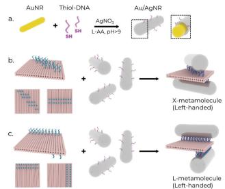
Fig. 2 Schematic showing the fabrication of the chiral metamolecules. (a) One-pot growth and functionalisation of the Ag shells on AuNRs. (b) and (c) Assembly of 'X' and 'L'-shaped chiral structures, respectively, constructed by varying the anchor configuration (blue strands) on the 2layer sheet DNA Origami (left). The 'upper' (left) and 'lower' (right) faces of the sheet are shown below the respective sheet structures
