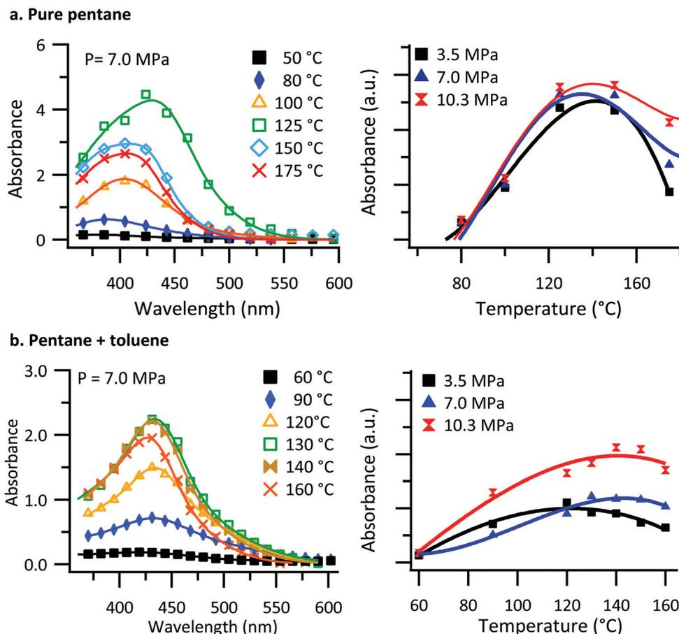
Fig. 1 *In situ* UV-vis transmission results of PBTTT-C<sub>14</sub> in (a) pure *n*-pentane and (b) *n*-pentane: toluene (0.5% mol) solution. UV-vis spectral measurements for the chamber and its contents (solution) for several temperatures and a single pressure (left) and the integrated UV-vis absorbance as a function of temperature for several pressures (right). Solid lines indicate the fit to the data using eqn (1).
