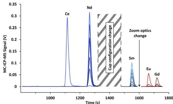
Fig. 7 Electropherogram obtained by CE-MC-ICP-MS for lanthanide fission products in a spent MOX fuel sample with a 120 mmol L<sup>-1</sup>  $\alpha$ -HMTA electrolyte. The signal break between 1300 and 1500 s was caused by a cup configuration change, while the shorter signal break between 1575 and 1625 s was due to a modification in zoom optics.
