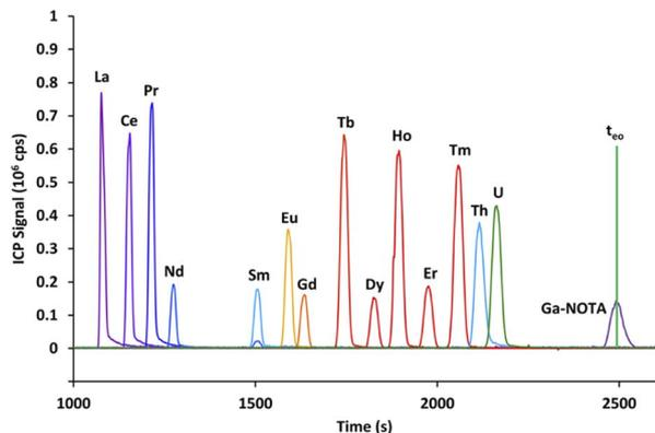
Fig. 2 Electropherogram obtained by CE-Q-ICP-MS for the mixture containing 14 lanthanides, uranium and thorium with a 100 mmol L<sup>-1</sup>  $\alpha$ -HMBA electrolyte. Here,  $t_{00}$  is the time where neutrals migrate, as calculated at the apex of the Ga-NOTA peak. Yb and Lu were omitted from the figure for visibility reasons.
