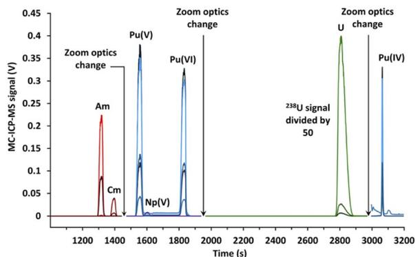
Fig. 6 Electropherogram obtained by CE-MC-ICP-MS for actinides in a spent MOX fuel sample with a 120 mmol L<sup>-1</sup>  $\alpha$ -HMBA electrolyte. The line breaks were caused by the change in zoom optics during the CE separation.
