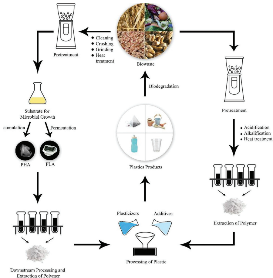
Fig. 5 Bioplastic production from renewable biowaste. Reproduced from ref. 120 with permission from Applied Biotechnology Research Center, Baqiyatallah University of Medical Sciences (BMSU), copyright 2021.
