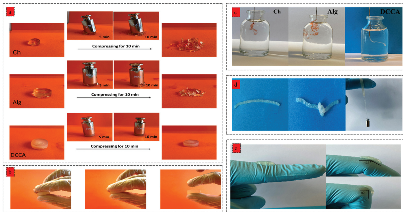
Fig. 4 (a) Deformation capability of Ch, Alg and DCCA hydrogels after being pressed by the 200 g weight for 10 min, and (b) deformation resistance of DCCA hydrogel by pressing between fingers, (c) injectability of Ch, Alg, and DCCA evaluation using a syringe with 30 G needles, (d) foldability and knotting ability of DCCA hydrogel and high mechanical flexibility could sustain a 50 g weight, (e) the DCCA hydrogel adherence to a knuckle which was repeatedly bent from 180° to 90° in the flexibility test 50 times to examine the flexibility and adhesion performance.
