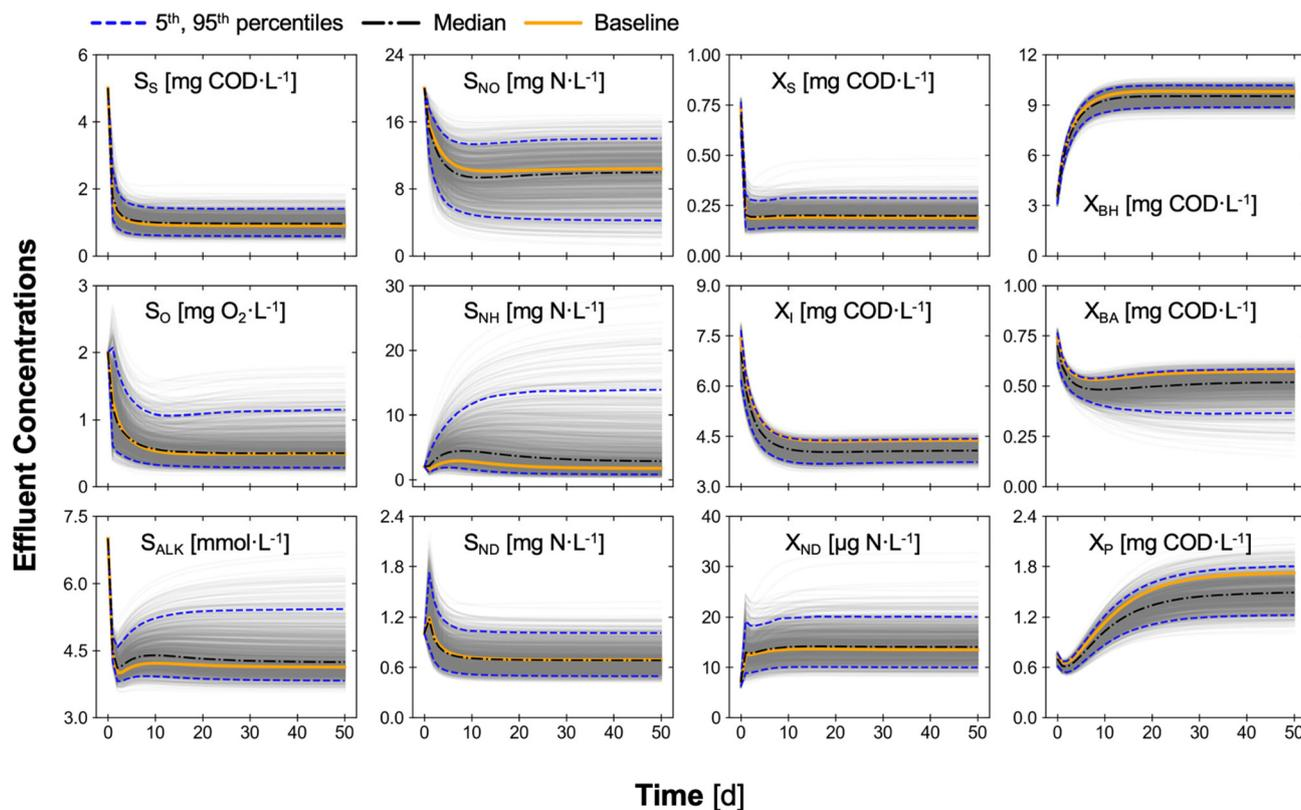
Fig. 5 Dynamics of the effluent state variables generated in Monte Carlo simulations of the BSM1 system for uncertainty analysis. Soluble inert organic matter,  $S_i$ , is omitted in this figure because it is not involved in any conversion processes, as defined in ASM1. Each solid grey line represents one sample. Median and 5th/95th percentiles at each time point were calculated based on the entire 1000 samples.
