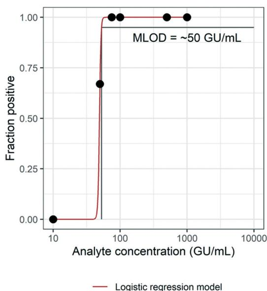
Fig. 3 Experimental estimation of the method limit of detection (MLOD) of the enhanced magnetic beads-based RNA extraction protocol using a logistic regression model ( $\beta_0 = -39.7$ ;  $\beta_1 = 0.8$ ) with a 95% limit of detection.
