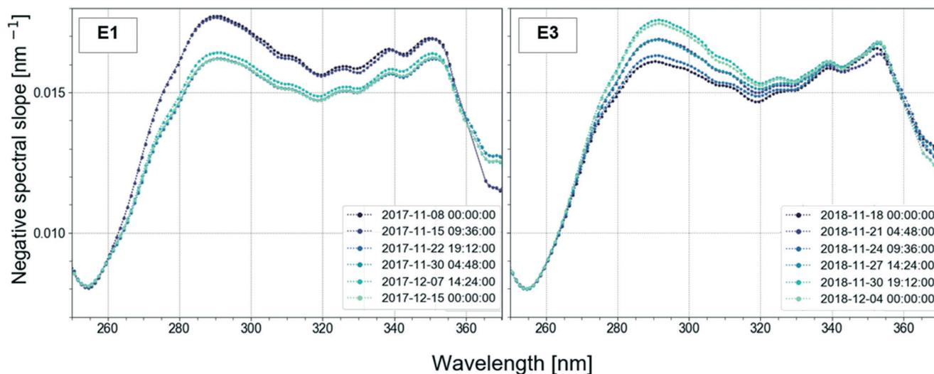
Fig. 5 Spectral slope curve of the spectro::lyser absorbance data in surface water as a function of wavelength calculated using the `abs_spectral_curve` function in the Abspectroscopy toolbox. The selected dates cover the period before, during and after the autumn lake circulation event in 2017 (left plot, November–December, event 1) and 2018 (right plot, November–December, event 3).
