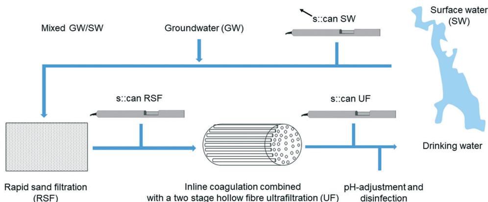
**Fig. 1** Treatment steps for the full-scale process at Kvarnagården DWTP, Varberg, Sweden, and placement of the three online spectrophotometers (spectro::lyser, s::can Messtechnik GmbH). The table is an example of the obtained fingerprint file with raw attenuation measurements [absorbance per meter] for a few wavelengths at 2.5 nm interval in the range 200–750 nm. The grab sampling locations coincide with the positions of the spectro::lyser units.
