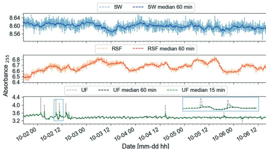
Fig. 3 Rolling median smoothing function with a 60-min window size applied on UV absorbance at 255 nm (absorbance per meter) time-series (October 2017) of surface water (SW), rapid sand filtrate (RSF) and ultrafilter permeate (UF). Comparison between specifying a window size of 60-min (black) vs. 15-min (green) in the function *rolling* in the AbspectroscOPY toolbox for the UF time-series, with a close-up showing narrow spikes in the light blue rectangle.
