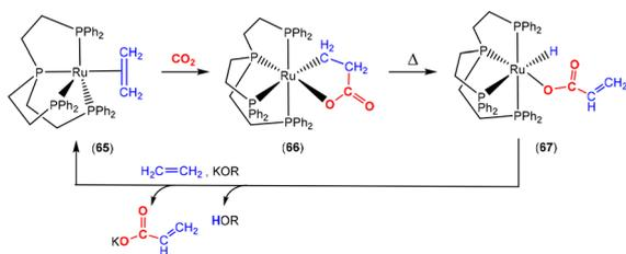
**Scheme 16** Investigations leading to the first example of the ruthenium-catalysed synthesis of acrylate salts from ethene and CO<sub>2</sub>.
