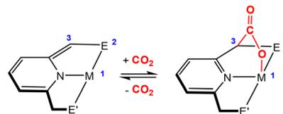
**Scheme 30** Generalised scheme highlighting the potential for reversible CO<sub>2</sub> activation *via* MLC involving dearomatisation–aromatisation. This is a 1,3-addition across a two-atom bridge.
