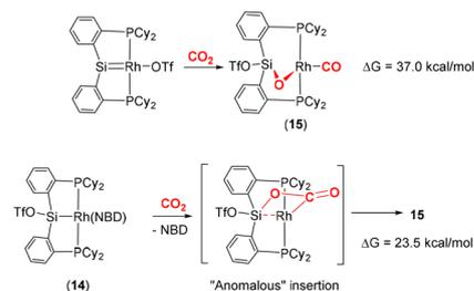
**Scheme 3** DFT calculated pathways for CO<sub>2</sub> reductive cleavage of CO<sub>2</sub> into CO and siloxide by complex 14. Top: silylene pathway, bottom: anomalous insertion pathway.
