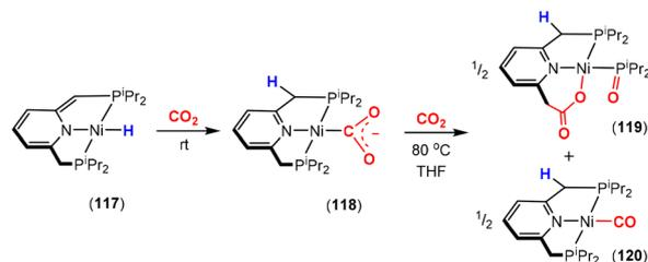
**Scheme 36** Reactivity of nickel–hydride pincer type complexes with CO<sub>2</sub> and subsequent transformation.
