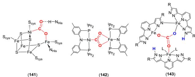
**Fig. 5** Carbon monoxide dehydrogenase C-cluster active site (**141**) found in the enzyme and its biomimetic model (**142**). Trinuclear iron complex **143** is the functional model of carbonic anhydrous.
