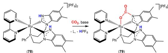
**Scheme 21** Activation of CO<sub>2</sub> by ligand cooperation on benzimidazole-based NHC complexes (L = weakly coordinating solvent ligand).
