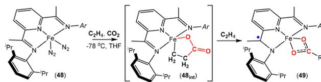
**Scheme 12** Unsaturated iron carboxylate products *via* proposed intermediate species **48<sub>int</sub>**. The R group is variable depending on the conditions (see text for details).
