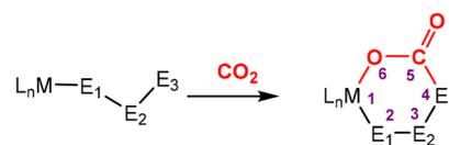
**Scheme 23** Schematic representation of the activation of CO<sub>2</sub> utilising a three-atom bridging unit (in some examples, an interaction between M and E<sub>3</sub> is possible).
