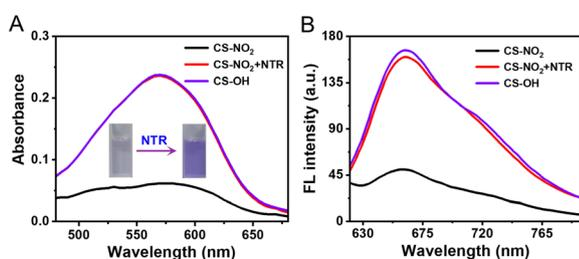
**Fig. 1** After 1 h of incubation at 37 °C, the (A) absorption and (B) fluorescence spectra of **CS-NO<sub>2</sub>** (10 μM) in the absence and presence of NTR (10 μg mL<sup>-1</sup>) with NADH (0.5 mM).  $\lambda_{\text{ex}}$  = 580 nm. Inset of (A): visible-light images of **CS-NO<sub>2</sub>** in the absence and presence of NTR.
