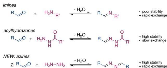
Fig. 1 Comparison between imines, *N*-acylhydrazones, and azines.
