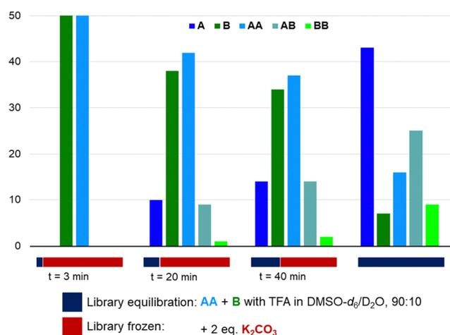
Fig. 4 The equilibration of a library starting from **AA** (14 mM) and **B** (14 mM) with TFA (14 mM) in DMSO-d<sub>6</sub>/D<sub>2</sub>O (90:10) can be brought to a halt by the addition of K<sub>2</sub>CO<sub>3</sub> (28 mM). The libraries were analysed by <sup>1</sup>H NMR spectroscopy after 5 hours, independent of the moment at which the library was frozen, and the results are shown in mol%.
