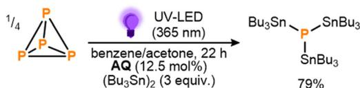
**Scheme 4** Optimized conditions for the direct, photocatalytic stannylation of  $P_4$  into  $(Bu_3Sn)_3P$  using anthraquinone (AQ) as photocatalyst. Stoichiometries in equiv. and mol% are defined per P atom.
