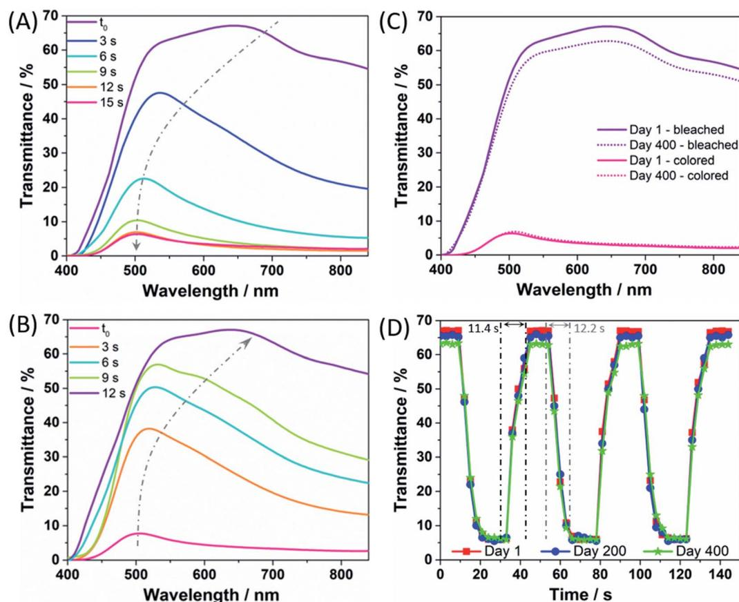
Fig. 3 Transmittance spectra for the PECD: (A) coloration process occurring under  $1000 \text{ W m}^{-2}$  (AM 1.5G) simulated sunlight and (B) bleaching process taking place under short-circuit and dark conditions. (C) Transmittance modulation of the PECD under bleached and colored conditions, comparing the spectra at day 1 and day 400 of the ageing test. (D) Transient transmittance response time for the PECD, comparing the traces at day 1, day 200 and day 400 of the ageing test.
