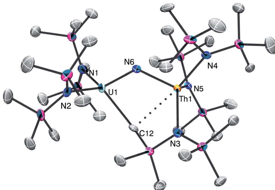
Fig. 2 Solid-state molecular structure of **3** shown with 50% probability ellipsoids. [K(18-crown-6)]<sup>+</sup> cation, [K(18-crown-6)(Et<sub>2</sub>O)<sub>2</sub>]<sup>+</sup> cation, and hydrogen atoms removed for clarity. Selected bond lengths (Å) and angles (°): U1–N6 = 2.002(4), Th1–N6 = 2.160(5), U1–N1 = 2.366(5), U1–N2 = 2.349(5), Th1–N3 = 2.389(5), Th1–N4 = 2.395(5), Th1–N5 = 2.408(5), U1–C12 = 2.525(6), Th1–C12 = 2.962(5), U1–N6–Th1 = 122.2(2).
